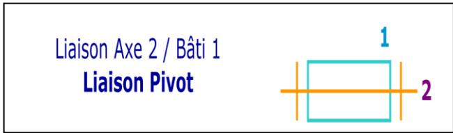
$$\begin{Bmatrix} R_x \\ 0 \\ 0 \end{Bmatrix} \begin{Bmatrix} 0 \\ 0 \\ 0 \end{Bmatrix} \quad \left\{ \tau_{M(2/1)} \right\} = \begin{Bmatrix} X \\ Y \\ Z \\ M \\ N \end{Bmatrix}$$
