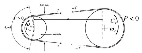
Entraxe:  $O_1O_2 = a$   $A_1A_2 = B_1B_2 = a.\cos \alpha$ Avec:  $\sin \alpha = \frac{R-r}{a}$   $A_1B_1 = r\theta_d = r(\pi - 2\alpha)$   $A_2B_2 = R\theta_D = R(\pi + 2\alpha)$
